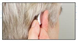
Pushing the Rocker Switch for about 2 seconds on either the upper or lower multi-control button will cause the program to change. Pushing the upper part of the switch advances the program to the next numerical program; the lower portion reverses the program direction. You will hear the same number of beeps (1, 2, 3, or 4) to announce the program you are in each time you press and hold the rocker switch.
